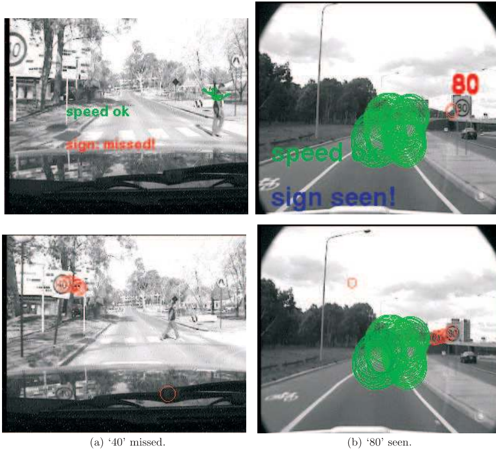
Fig. 21. The two columns are typical cases for the speed sign inattention system when the vehicle was not speeding. (a) The system detected that the driver most likely missed the road sign. (b) The driver most likely observed the sign. Top row: Live video feeds showing current view, eye gaze (dots/large circles) and current status (overlaid text) during screen-shot. Bottom row: Last detected signs (small circles) and eye gaze during detection (dots/large circles). The small circles on the hood and in the sky in the bottom row are due to a rendering bug at the time of test. They coincide with stale returns that had a strong momentary circular return but failed classification.
