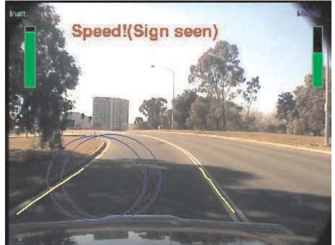
Fig. 32. Screen-shots of the Automated Co-driver. Vehicle speeding, although last speed sign was observed by the driver. Large circles: driver gaze.
