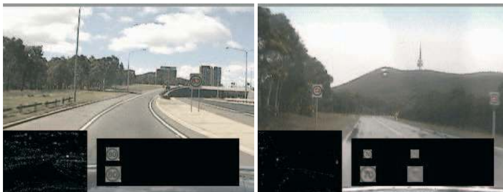
Fig. 10. Sign detection using Fast Radial Symmetry Transform (FRST). The bottom left corner shows the FRST image, where the red crosses highlight detected signs.
