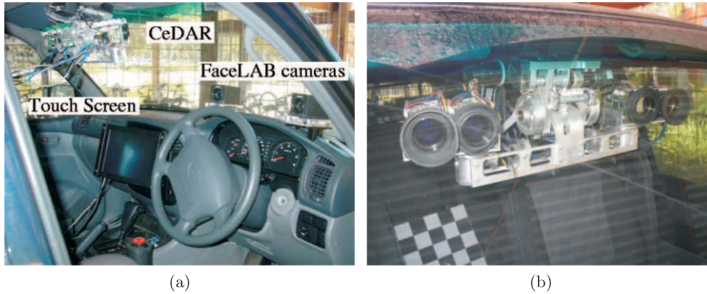
Fig. 6. (a) The cameras on-board the vehicle. The CeDAR active vision platform containing the stereo road scene cameras and faceLAB TM passive stereo cameras observing the driver. (b) CeDAR: Cable Drive Active vision Robot in vehicle. Four cameras are arranged in two stereo pairs. Cameras are fitted with polarizing filters and far-field cameras use glare hoods.
