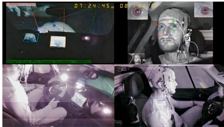
Figure 3. Four different views of the driver and the test track. These views were observed thoroughly by an expert to define a ground truth for driver drowsiness based on drowsiness signs into three classes (informed consent was obtained from the driver to publish his image in this paper; reprinted from our previous study [2], license no. 5218171384545).
