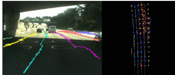
(c) Shadows continue to pose a natural challenge for lane detection systems.
