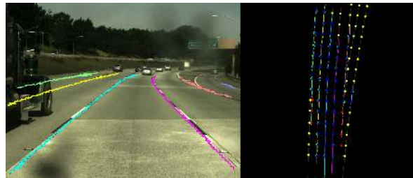
(b) Labels from TagEval reveal that the network is weak at capturing lanes in scenarios with off-ramps. However, note that on the left, the network is able to make lane detections even in the presence of the occluding truck.
