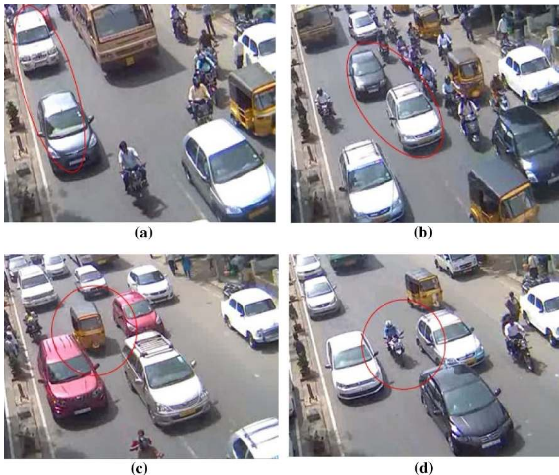
Fig. 10 Following behaviors in mixed traffic. a Car following, b staggered following, c following between two vehicles, d passing
