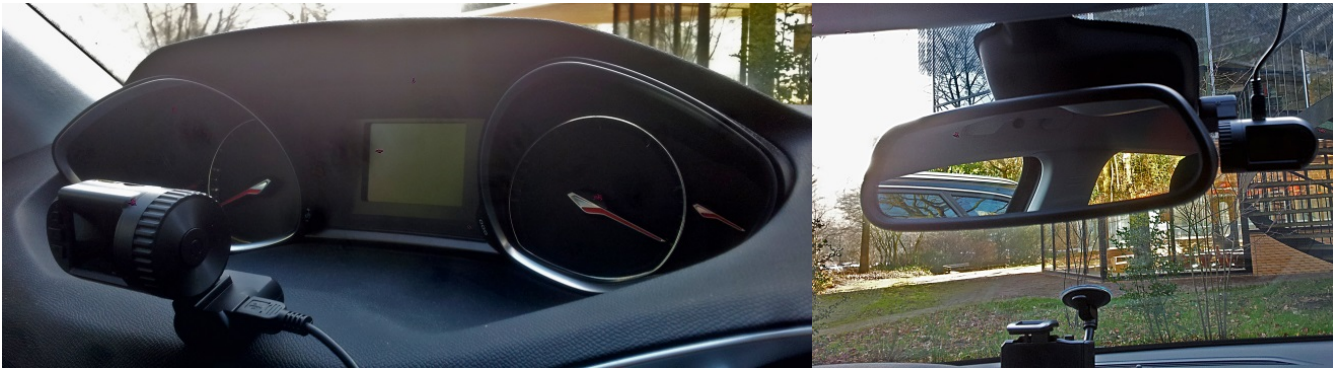
Fig. 1. Installed cameras, pointed at the dashboard (left) and behind the rear-view mirror (right).
