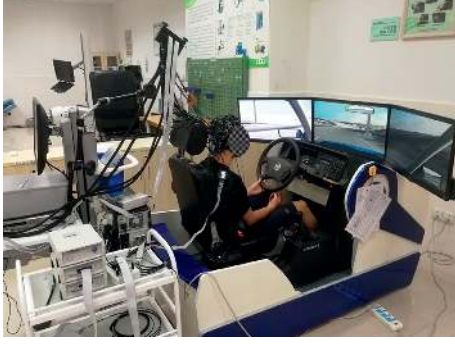
FIGURE 2: The setup of the experiment, including the driving platform and EEG recording system.
