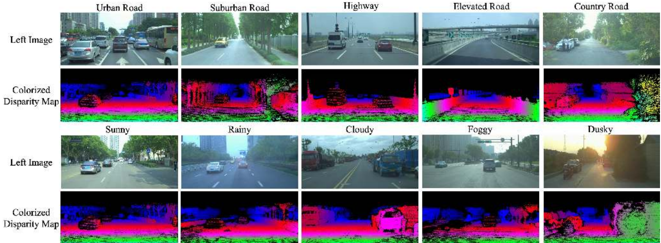
Figure 1. Examples of our DrivingStereo dataset. Our dataset contains a diverse range of driving scenarios. The image of the left camera and the disparity map are shown.
