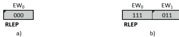
Figure 5. RLEP encodes the number of symbols in the run where each EW consists of 3 bits in this example and a) contains one EW set to 0 indicating that the run-length indicated by this EW_0 is 7 (refer Table 1) and that no other EW will be concatenated, b) the RLE Packet consists of two EWs, the first EW_0 is set to 7 and encodes a run-length of 7 while indicating that one more EW will follow. This EW_1 is set to 3 and therefore the run-length encoded by this EW is 3. At the same time, it indicates that no further EW will follow in a given RLEP.
