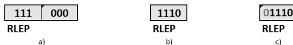
Figure 6. Run-length encoding with the number of symbols 14 while selecting different lengths of EWs where a) the EW length set to 3 requires the concatenation of two EWs which means the use of overall 6b b) the use of an EW with a length of 4b allows optimal encoding and c) using an EW with the length of 5b means unnecessarily long bit sequence with one leading 0.
