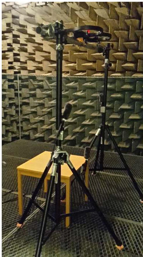
Figure A.1: Cyclone in the anechoic chamber. Figure A.2: X4 in the anechoic chamber.
