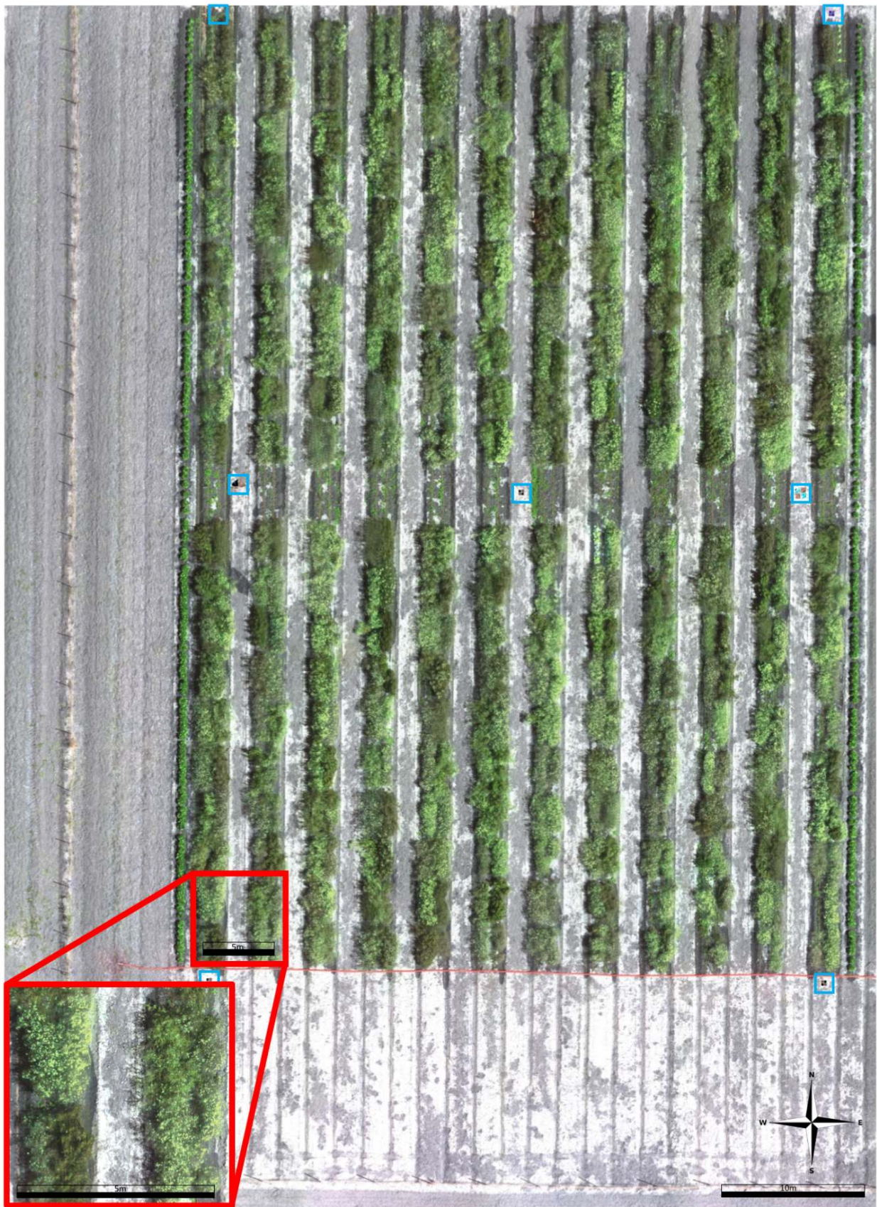
Figure 2. Reconstructed field orthomosaic image at 11:00 am on July 1 st , 2019. A total of 2,355 raw drone images in five reflectance bands (red, blue, green, red-edge and infrared) were tiled using the Pix4Dmapper Pro software in GPS-guided mode. Only the red, blue and green channels are shown in this figure. The seven ground control points are identified with blue boxes.
