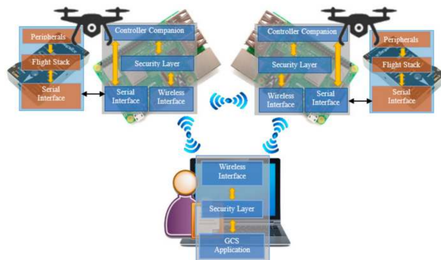
Figure 8. An illustration of UAV ad-hoc network architecture implemented in the experimental simulation.
