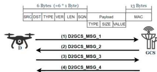
Figure 2. D2GCS communication and packet structure.
