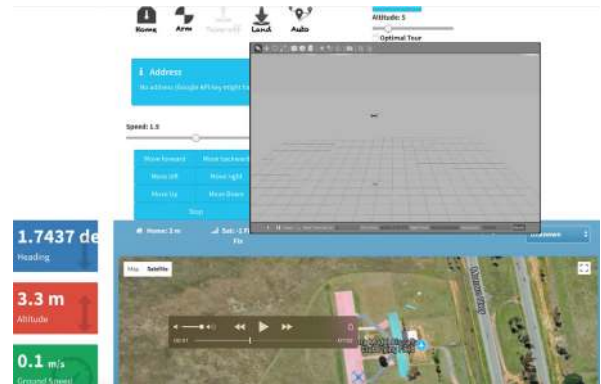
Fig. 9. Control of Gapter using ROSLink with SITL and Gazebo Simulators.
