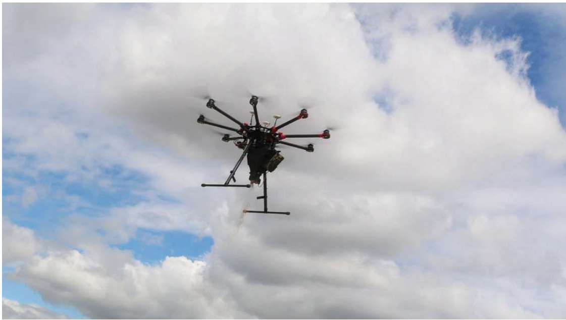
Fig. 5. Prototype of BugBot predatory mite dispenser. BugBot, developed by mechanical and aerospace engineering students at the University of California Davis, is a drone-mounted dispenser that can distribute predatory mites, important biological control agents of spider mites. In the picture, the BugBot dispenses vermiculite, the mineral substrate the predators can be obtained in.
