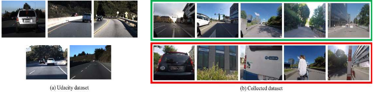
Fig. 3: (a) Udacity images used to learn steering angles. (b) Collected images to learn probability of collision. The green box contains no-collision frames, and the red one collision frames.
