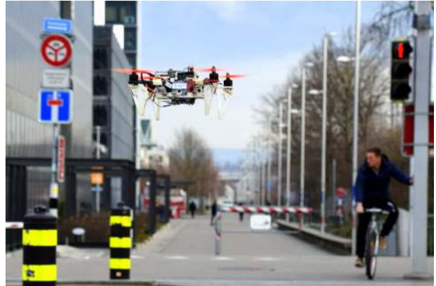
Fig. 1: DroNet is a convolutional neural network, whose purpose is to reliably drive an autonomous drone through the streets of a city. Trained with data collected by cars and bicycles, our system learns from them to follow basic traffic rules, e.g. do not go off the road, and to safely avoid other pedestrians or obstacles. Surprisingly, the policy learned by DroNet is highly generalizable, and even allows to fly a drone in indoor corridors and parking lots.
