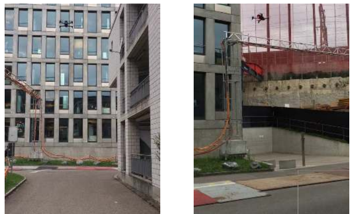
Fig. 6: High altitude Outdoor 1: In order to test the ability of DroNet to generalize at high altitude, we made the drone fly at 5 m altitude in the testing environment Outdoor 1 . Table II indicates that our policy is able to cope with the large difference between the viewpoint of a camera mounted on a car (1.5 m) and the one of the UAV.
