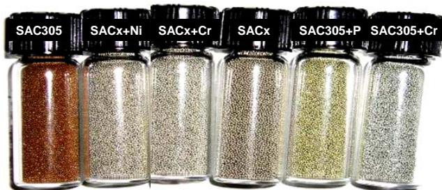
FIGURE 21: Effect of alloy additives on the tarnish resistance of solder spheres. (12 Hrs aging at 125°C; 168Hrs at 85%RH and 85°C; 3x reflow in air at 255°C for 30 sec TAL)
