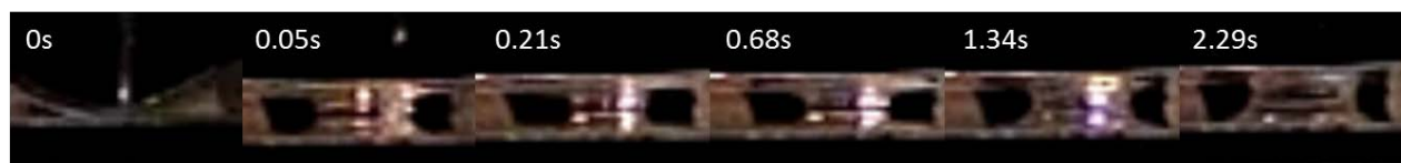
Fig. S1 Snapshots of the droplet relaxation process, recovering to a unstressed state from being deformed.
