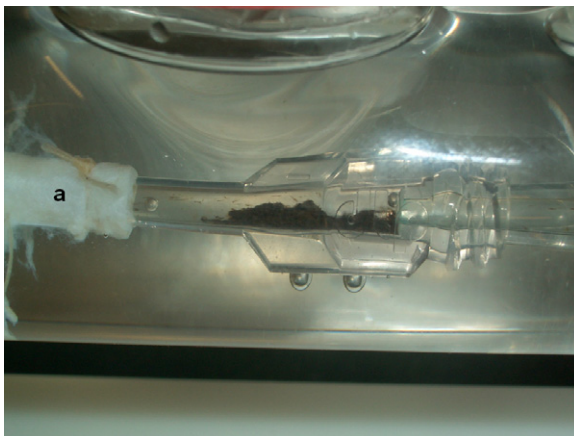
Figure 9. Artery model: a precipitate of nanoparticles in the circuit after the application of magnetic force at the outlet of the artery (a).
