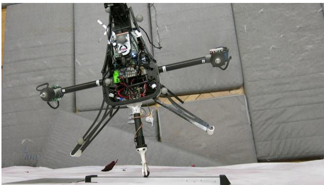
Fig. 16. A top-down view of the UAV scanning across the stepped aluminum bar. This was captured during the second of two passes completed within a continuous contact interaction; traversing from left to right to left as pictured.
