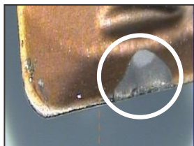
Fig. 19 Cutting edge chipping localisation
