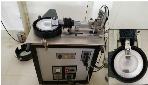
Fig. 8 The experimental set up of pin-on-disc wear test
