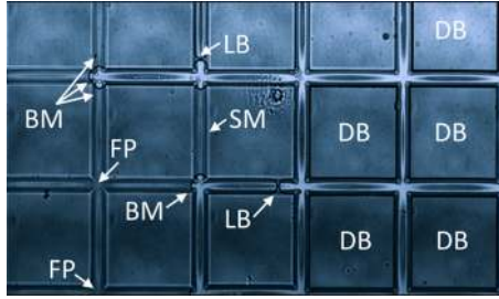
Fig. 8 A tile scan of the drying pore network shows the vicinity of pore junctions evidencing the representative phenomena occurring during the drying process: full or saturated pores (FP), empty pores (all other pores in the figure, not denoted), bulk menisci (BM), single menisci (SM), liquid bridges (LB) as well as completely dried throats (surrounding the denoted dried blocks (DB) in the figure) and throats containing liquid rings (all other throats)
