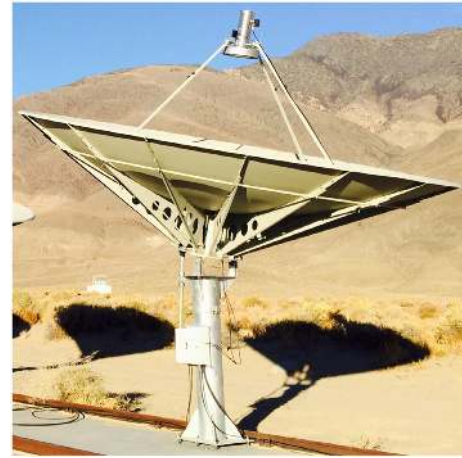
Figure 2. An example of an assembled DSA-10 dish, with the receiver mounted. The dish is 4.5 m in diameter, formed of 16 separate aluminium panels, with a surface accuracy of < 0.5 mm.
