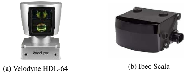
Figure 2: LIDAR sensors mounted on our data collection vehicle. Left: Velodyne HDL-64 LIDAR which costs $75,000. Right Ibeo Scala Lidar which is priced at $1000. Note that the Velodyne has 16x more vertical resolution than the Scala.
