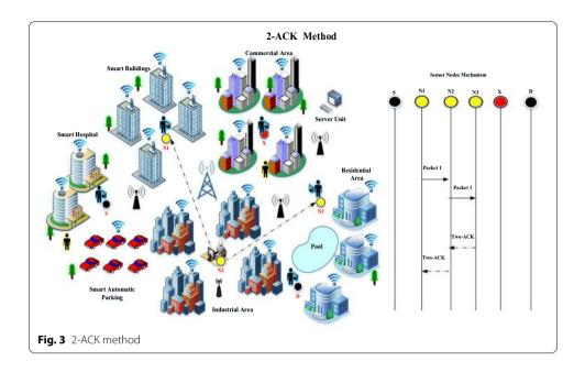
Suppose three consecutive nodes (triplet) alongside a path are N1, N2, and N3. Node N1 will deliver packet 1 to N2, and N2 will deliver the same to N3.
