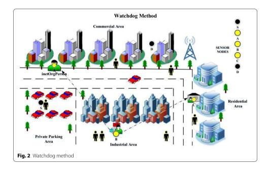
The above-described method can be better understood with the block diagram of Fig. 2. It detects the misbehaving nodes [11]. Suppose a path runs from node S to D through A, B, and C. Still, A is not capable of transmitting to C, but it can respond to B. So, A can tell if B broadcast the packet. If encryption is not conducted on each connection (which itself is an expensive and complex affair), then A can also say whether B has tampered with either payload or header.
