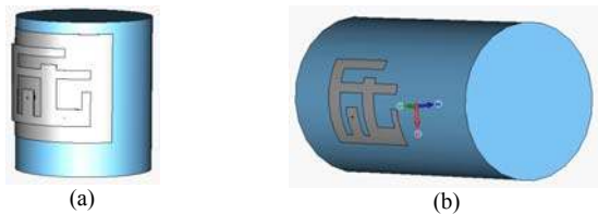
Fig. 6. Antennas bent around cylinders for different directions: (a) E-plane direction and (b) H-plane direction.
