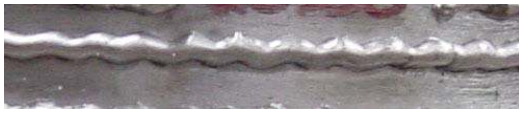
Figure 5-6-5, Weld bead and cross section view of DB-GMAW (Bypass current L&R : 50A-50A)
