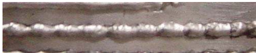
Figure 5-6-3, Weld bead and cross section view of DB-GMAW (Bypass current L&R : 40A-40A)
