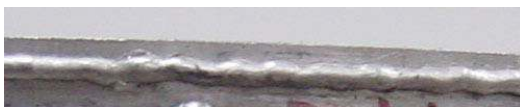
Figure 5-6-4, Weld bead and cross section view of DB-GMAW (Bypass current L&R : 45A-45A)
