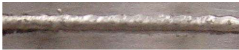
Figure 5-6-2, Weld bead and cross section view of DB-GMAW (Bypass current L&R : 30A-30A)
