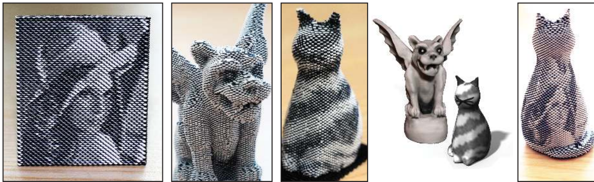
Figure 1: Left: Lena image 3D printed on a MakerBot Replicator 2X. This plate is 3.5 cm tall and about 2 mm thick. We achieve approx. 50 dpi vertically with a 60×71 texture modulated on 142 alternating black and white layers. Center: 3D models printed with continuous tone. Corresponding texture maps: an ambient occlusion texture gives the GARGOYLE (10.2 cm tall) an aged appearance while we fit LUCYCAT (5.4 cm tall) with a calico coat. Right: the Lena texture remains sharp after projection.
