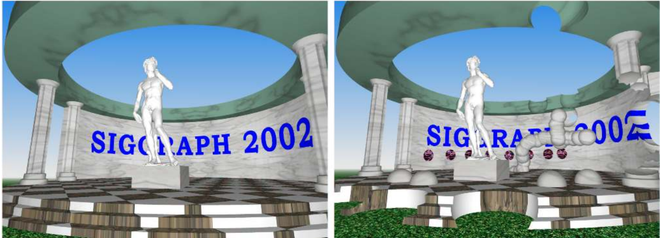
Figure 1: A temple undergoing destructive modifications. Both models were generated by dual contouring a signed octree whose edges contain Hermite data. The modified model on the right was computed from the lefthand model in real-time.
