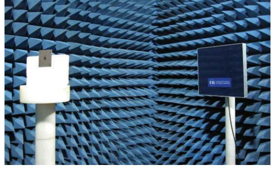
FIGURE 10: Measurement environment of the tag.
