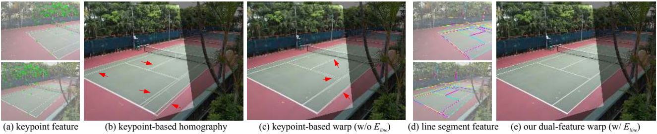
Figure 6. Comparison of mesh-based homographies estimation used in image registration. Misalignments are illustrated by red arrows.
