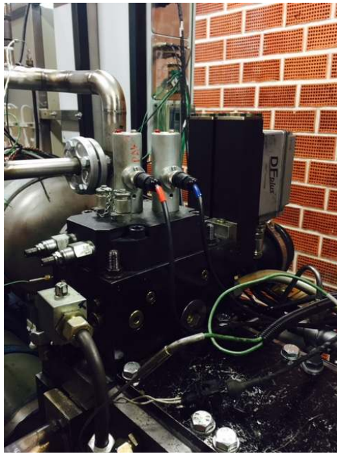
Figure 13. EHVA control solenoids
