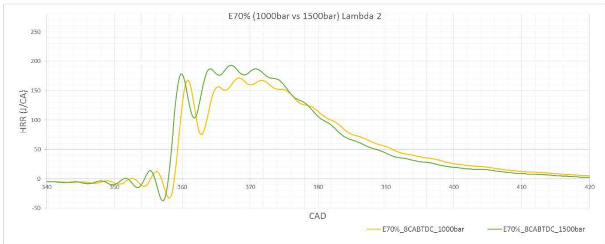
Figure 29. HRR figures of E70% conditions with diesel pilot injection pressure as a variable
