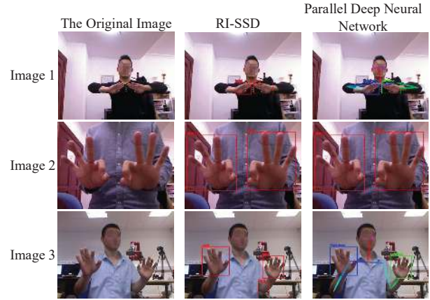
Fig. 10. For image 1, the RI-SSD and parallel network can both detect and locate both hands, but the parallel network can also distinguish between the right and left hands. For image 2, when the hands are too large for estimating the human body pose, the parallel network can only detect the two hands as a hand. For image 3, RI-SSD generates an incorrect detection, but the parallel network can remove this incorrect detection.
