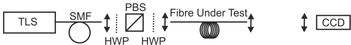
Figure 4: Experimental set-up for measuring the power transfer between the two cores in the DHC-ARF using a tuneable laser source (TLS) coupled via a single mode fibre (SMF), lens arrangement and polarization control (HWP: half wave plate, PBS: polarizing beam splitter) into the fibre under test (DHC-ARF). The output of the fibre under test is recorded on a CCD camera.
