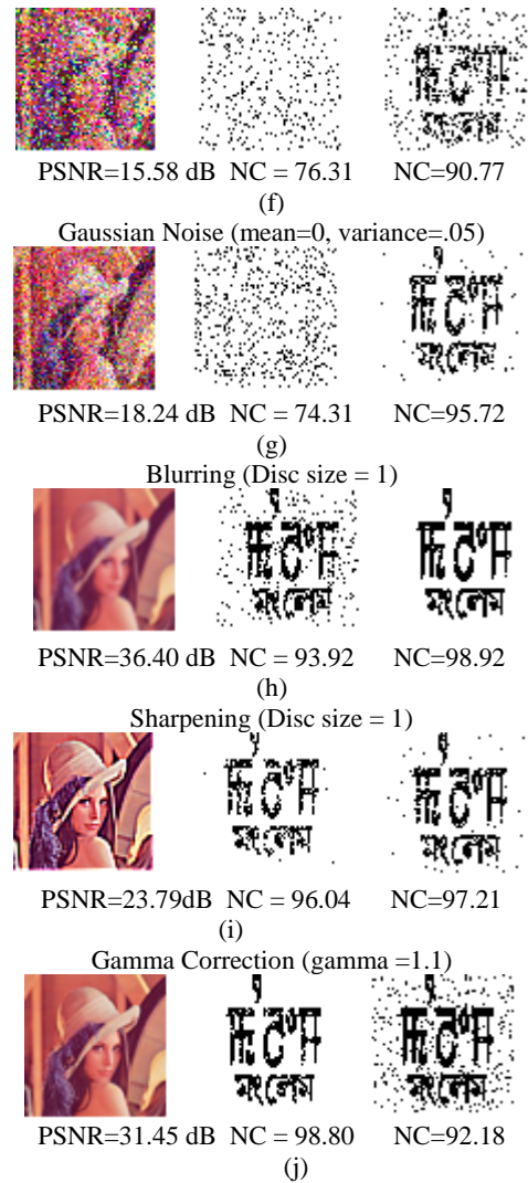
Fig6: Extracted watermarks from attacked watermarked image under various attacks.
