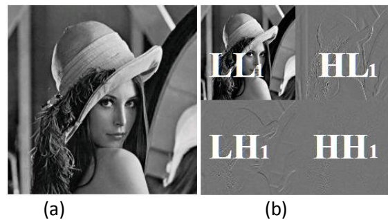
Fig 1: The original image (a) is divided into 4 sub bands (b) through 1-scale level wavelet transformation.
