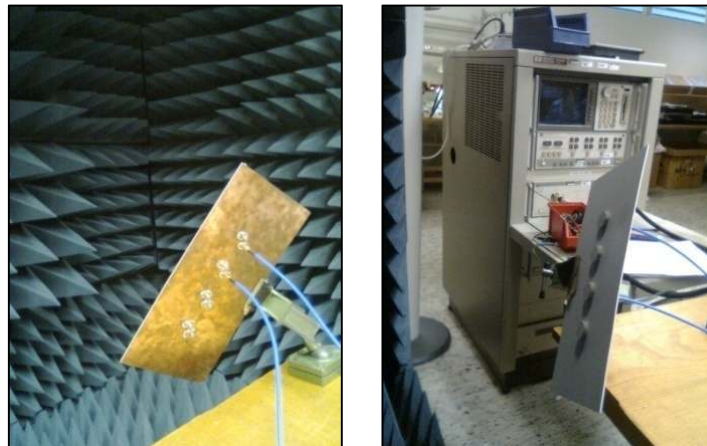
Figure 73: Two-port measurement of the 4\times 1 array antenna. The resonators are directed to an absorbing wall to avoid radiation scattering effects. The antenna is seen on face of the ground plane and the coaxial connectors (left); view of the resonator face with the network analyzer in the background (right).
