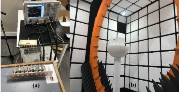
Fig. 16. Prototype of the proposed linear array and detailed illustration for measurement.
