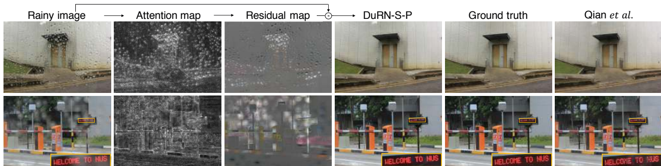
Figure 12: Examples of raindrop removal along with internal activation maps of DuRN-S-P. The “Attention map” and “Residual map” are the outputs of the Attentive-Net and the last Tanh layer shown in Fig. 13; they are normalized for better visibility.
