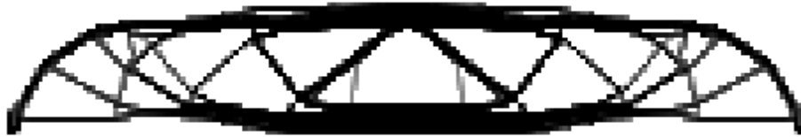
(b) Result for m = 6 : f_v = 0.353 , f_c = 311.09 , N_{act} = 94 , n_{[1]} = 565 , n_{[i]} = 482 , \phi_{B\&W} = 0.821 , T_{avg}^I = 229.4 , N_{iter} = 99 , n = 2700
