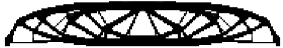
(d) With stress con. m = 6 : f_v = 0.50 , f_c = 196.09 , N_{act} = 27 , n_{[1]} = 1299 , n_{[i]} = 56 , \phi_{B\&W} = 0.979 , T_{avg}^I = 408 , N_{iter} = 74 , n = 2700
