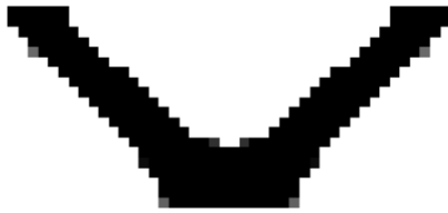
(c) No stress con. m = 4 : f_v = 0.235 , f_c = 220.83 , N_{act} = 1 , n_{[1]} = 276 , n_{[i]} = 8 , \phi_{B\&W} = 0.993 , T_{avg}^I = 0.0 , N_{iter} = 50 , n = 1200
