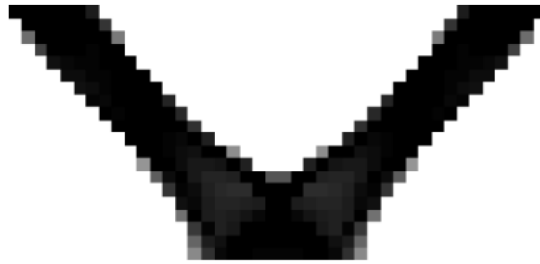
(a) Result for m = 4 : f_v = 0.234 , f_c = 233.81 , N_{act} = 144 , n_{[1]} = 106 , n_{[i]} = 196 , \phi_{B\&W} = 0.837 , T_{avg}^I = 6.7 , N_{iter} = 26 , n = 1200
