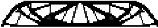
(a) No stress con. m = 4 : f_v = 0.50 , f_c = 189.69 , N_{act} = 1 , n_{[1]} = 543 , n_{[i]} = 67 , \phi_{B\&W} = 0.944 , T_{avg}^I = 0.0 , N_{iter} = 45 , n = 1200
