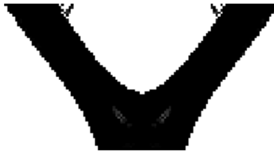
(g) With stress con. m = 12 : f_v = 0.25 , f_c = 202.07 , N_{act} = 71 , n_{[1]} = 2588 , n_{[i]} = 120 , \phi_{B\&W} = 0.989 , T_{avg}^I = 3714 , N_{iter} = 95 , n = 10800
