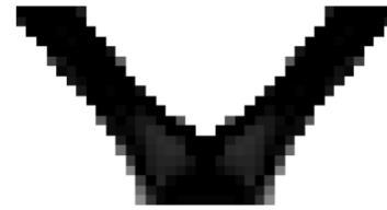
(d) With stress con. m = 4 : f_v = 0.237 , f_c = 233.5 , N_{act} = 147 , n_{[1]} = 128 , n_{[i]} = 174 , \phi_{B\&W} = 0.855 , T_{avg}^I = 12.30 , N_{iter} = 102 , n = 1200
