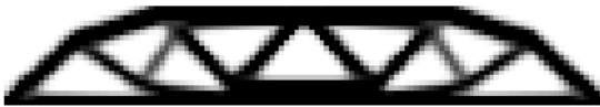
(e) With filter. m = 4 : f_v = 0.50 , f_c = 196.65 , N_{act} = 7 , n_{[1]} = 408 , n_{[i]} = 569 , \phi_{B\&W} = 0.526 , T_{avg}^I = 18.95 , N_{iter} = 250 , n = 1200
