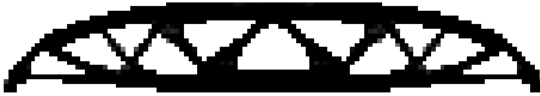
(c) With stress con. m = 4 : f_v = 0.50 , f_c = 194.31 , N_{act} = 3 , n_{[1]} = 564 , n_{[i]} = 41 , \phi_{B\&W} = 0.966 , T_{avg}^I = 101 , N_{iter} = 54 , n = 1200
