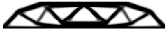
(f) With filter. m = 6 : f_v = 0.50 , f_c = 196.49 , N_{act} = 17 , n_{[1]} = 935 , n_{[i]} = 1210 , \phi_{B\&W} = 0.552 , T_{avg}^I = 139.98 , N_{iter} = 250 , n = 2700
