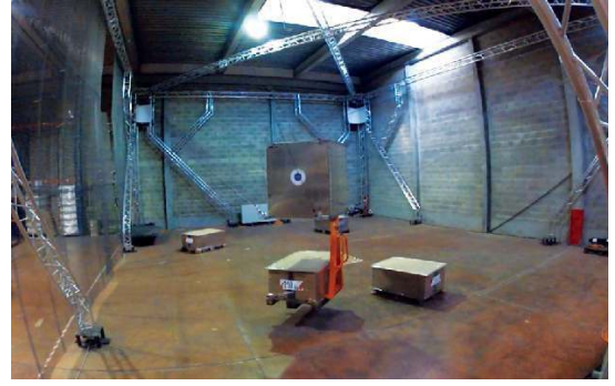
Fig. 2. The LIRMM/Tecnalia COGIRO suspended CDPR prototype.
