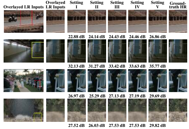
Figure 5: Visual comparisons of results from different training stages of the proposed framework. Please see Table 2 for the specific setting of each model variant. PSNR values are provided below the corresponding output frames.
