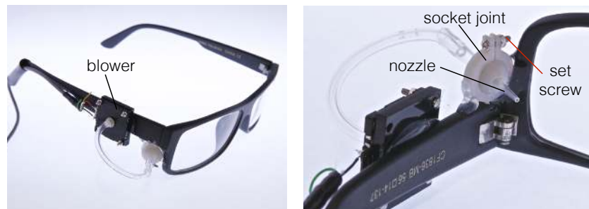
Fig. 6. Glasses with the air puff, that were used in the user study. A close up of the nozzle assembly is shown on the right.
