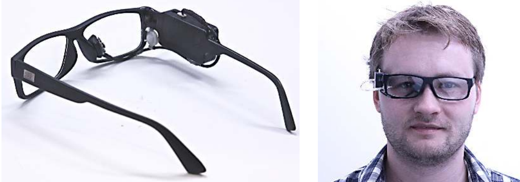
Fig. 1. Prototype with electronics integrated into the frame. This prototype is worn on the right image.
