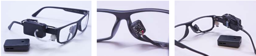
Fig. 2. Prototype that clips on the existing frame. Left image: prototype is shown next to the removable box that houses the electronics. Middle: a close-up of the IR sensor. Right: The prototype screws into the frame using an adapter on the back.
