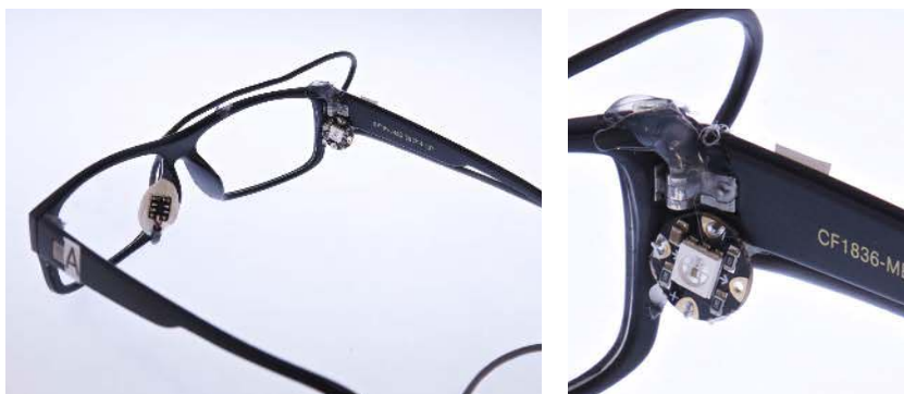
Fig. 4. Glasses with an LED light flash. The whole frame is shown on the left. A close-up of the LED is shown on the right.
