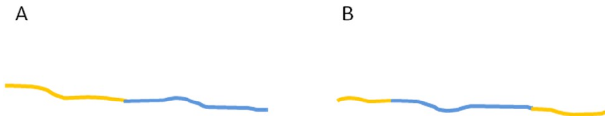
Figure 1. Schematic representation of amphiphilic copolymers AB (A) and ABA (B) Copolymers , where the hydrophobic block is represented in blue and hydrophilic block in yellow.
