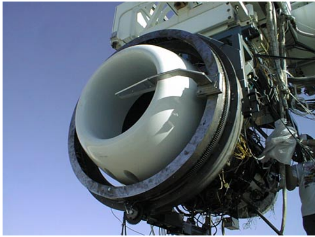
(a) Photographs of inlet rake installed on TFE731-60 engine
