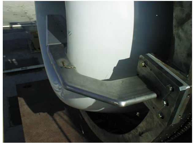
(a) Photographs of inlet rake installed on TFE731-60 engine
