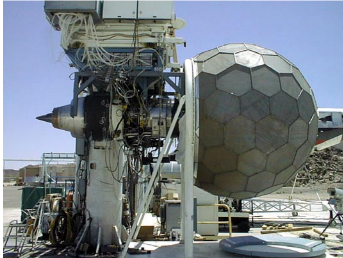
(a) Photograph of TFE731-60 engine on Honeywell test stand
