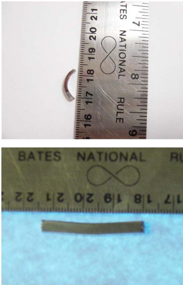
FIG. 4 (color online). (a) A 1.8 \text{ mm} \times 3 \text{ mm} \times 15 \text{ mm} bar shaped \text{Pt}_{57.5}\text{Cu}_{14.7}\text{Ni}_{5.3}\text{P}_{22.5} sample bent over a mandrel of radius 6.35 mm. The strain to failure exceeds 14.2%. (b) \text{Pt}_{57.5}\text{Cu}_{14.7}\text{Ni}_{5.3}\text{P}_{22.5} samples with dimensions of 4 \text{ mm} \times 4 \text{ mm} \times 34 \text{ mm} bent over a mandrel with a radius of 6 cm. The strain to failure exceeds 3%.
