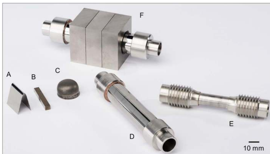
Fig. 1. Overview of the material system “tungsten laminated composites”. The starting point is severely cold-rolled tungsten foils (A) that are joined together into a multilayer material (B, Charpy impact test sample, 3 mm × 4 mm × 27 mm, 1 mm notch, KLST type). Three-dimensional shapes such as a cap (C) or a pipe (D, E) can be produced. The pipes are used as structural tungsten in high heat flux test components (F).
