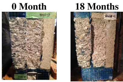
(a) Concrete cohesion failure
