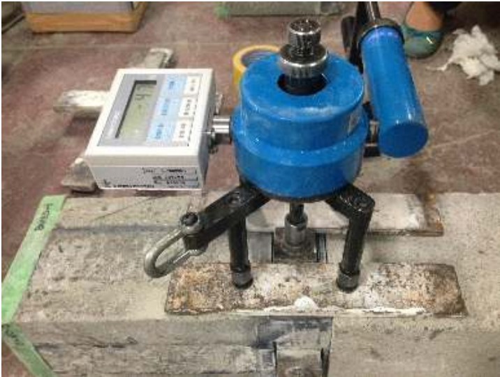
Fig. 6. Direct pull-off test setup
