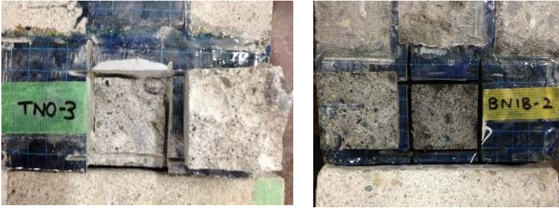
Fig. 20. Comparison of typical failure mode before and after 18 months of exposure
