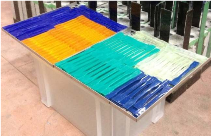
Fig. 1. Epoxy resin specimens for the tensile test
