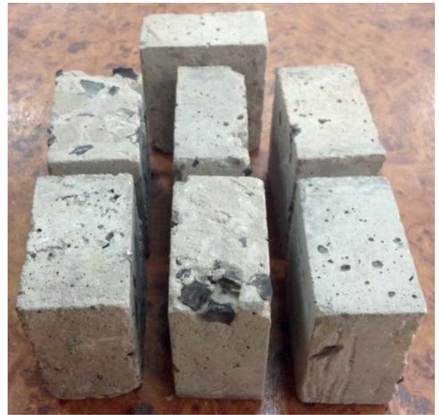
Fig. 5 Specimens of lightweight concretes after 100 freeze-thaw cycles
