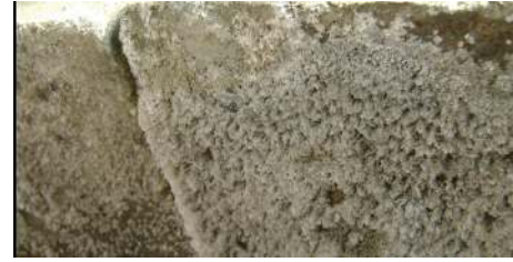
FIGURE 5: White deposits on geopolymer specimens exposed to magnesium sulphate solution.
