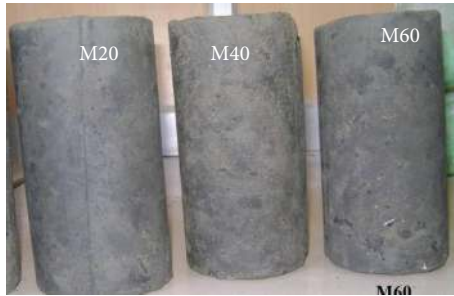
FIGURE 3: Geopolymer specimens exposed to 5% magnesium sulphate solution.
