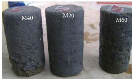
FIGURE 4: Geopolymer specimens exposed to 2% sulphuric acid solution.
