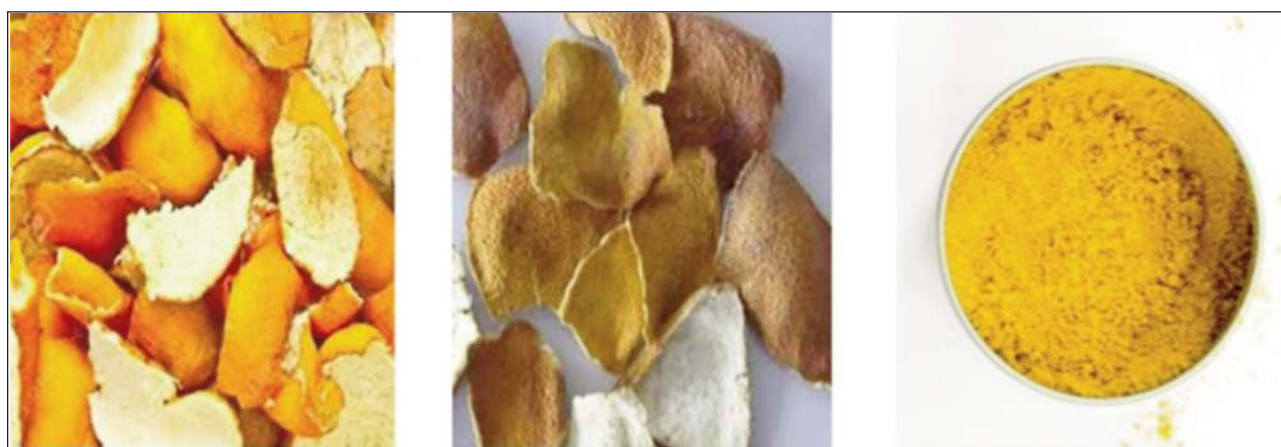
Fig. 1. Preparation of orange peel raw material: a – washed orange peel; b – dried orange peel; c – orange peel powder
