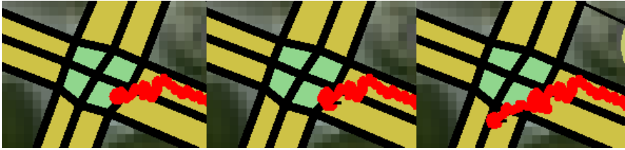
Figure 8.8: An example where noise makes it look like a car enters a crossing twice. Each red dot is an observed car position.
