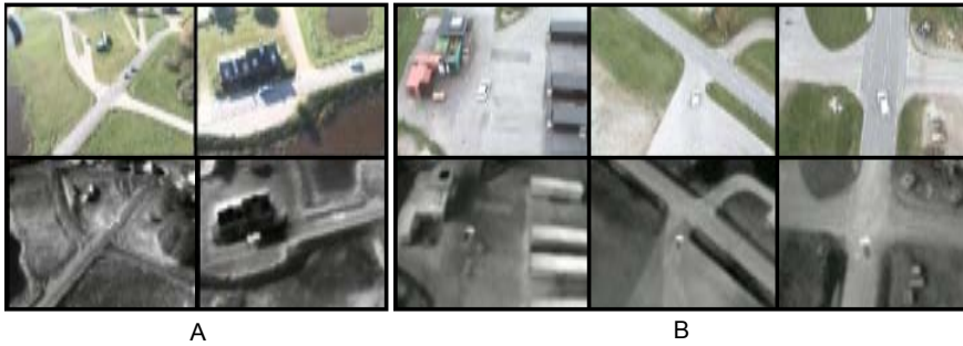
Figure 8.7: A. Two frames from a video sequence with the UAV hovering close to a road segment observing two cars performing an overtaking maneuver. B. Three frames from a video sequence with the UAV following a driving car passing road crossings. The top row contains color images and the bottom row contains corresponding thermal images.
